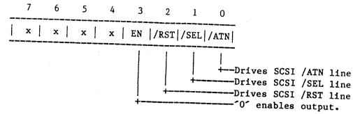
Notes: With GM849 bits 0-2 directly drive the appropriate SCSI line. They are only active for the duration of the write cycle.
