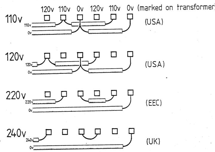
IN ALL CASES THE EARTH WIRE MUST BE CONNECTED TO THE EARTH TAG IMMEDIATELY BELOW THE ROW OF PRIMARY TERMINALS.
